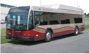
Manufactured by Gillig LLC, the new buses have a BAE Hybrid Drive system. The BAE Hybrid bus is expected to produce a fuel economy improvement of 30%. The maintenance cost to operate the bus will be reduced due to a smaller engine, no belts, no starter, no hydraulic components and a self-contained air conditioning system. The oil change interval of the engine can now be extended due to the reduction in the Red Rose Access
