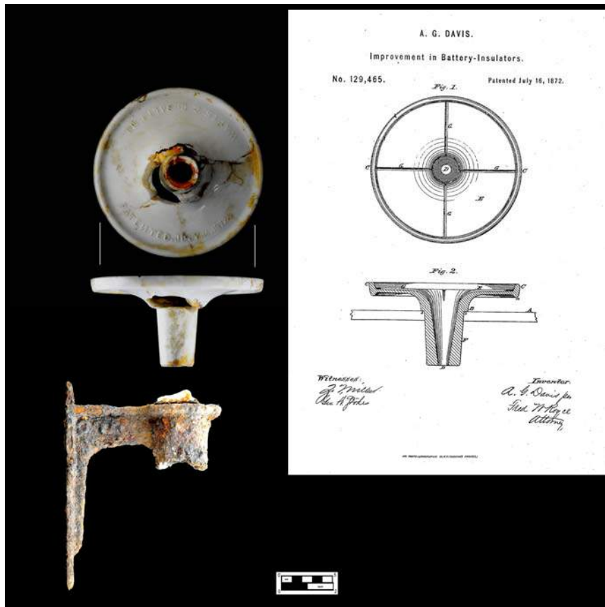
Figure 6.46 Watts patented telegraph insulator and iron bracket. (Top left) two views of opaque glass Watts insulator patented July 16, 1872. (Cat. 65.2); (bottom left) side view of iron bracket with insulator fragments attached; (right) A.G. Davis patent for "Improvement in Battery-Insulators" patent number 129,465 (Cat. 65.18).
